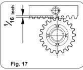
• Do not use grease or other lubricants between rack and pinion.
